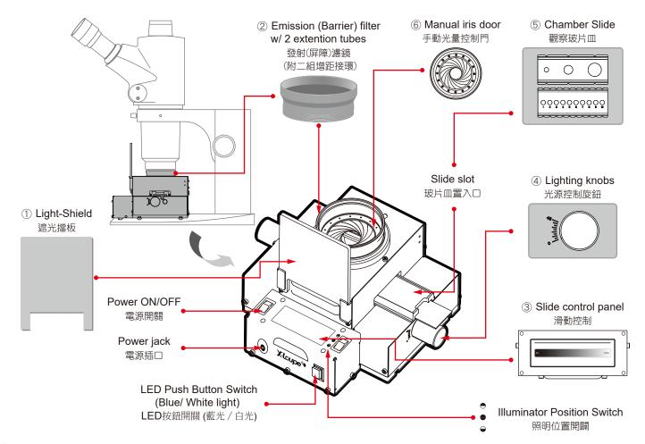
① UV/ Blue light Shield is designed with trigger function for protection to avoid the leak of blue light to damage eyes. 遮光擋板具有起動保護功能設計,以避免洩漏的藍光,對眼睛造成損害。
